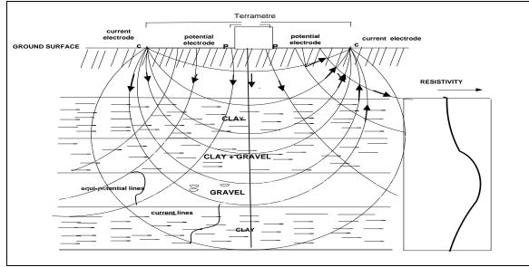
Fig. 2 Setting of electrodes spacing
