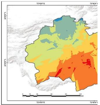
Fig. 5 Groundwater probability map using resistivity survey
