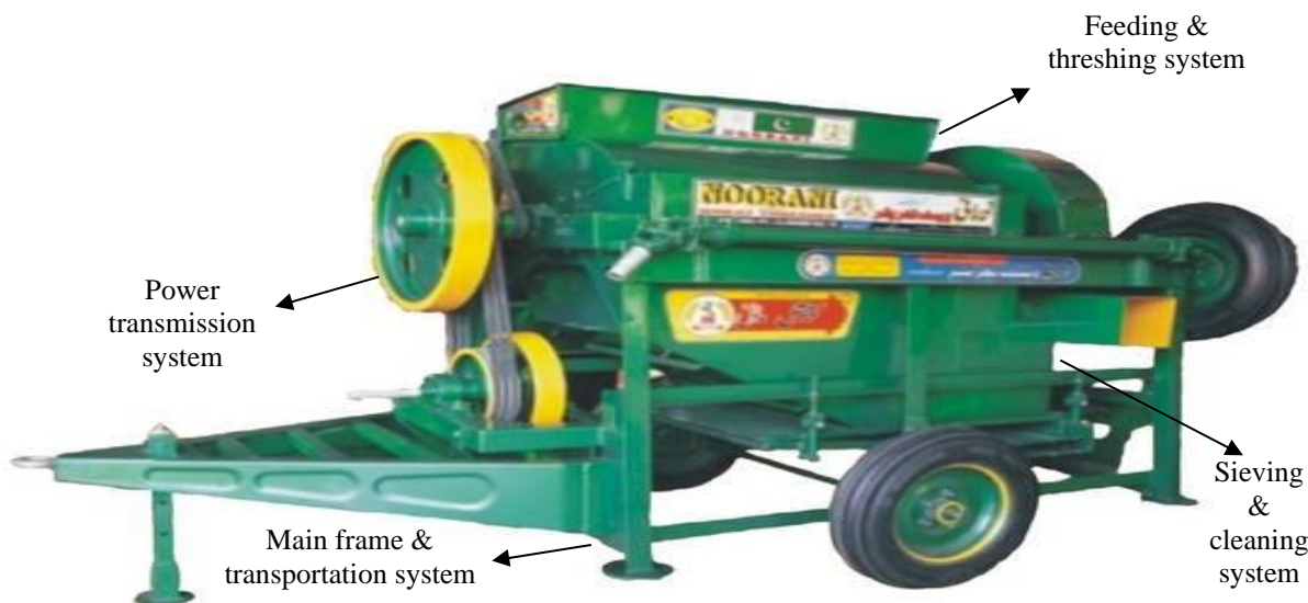
Fig. 1 Wheat thresher and its functional units
