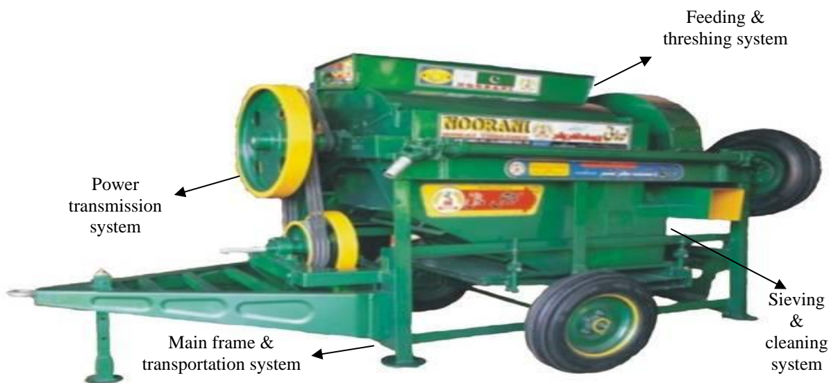
Fig. 1 Wheat thresher and its functional units
